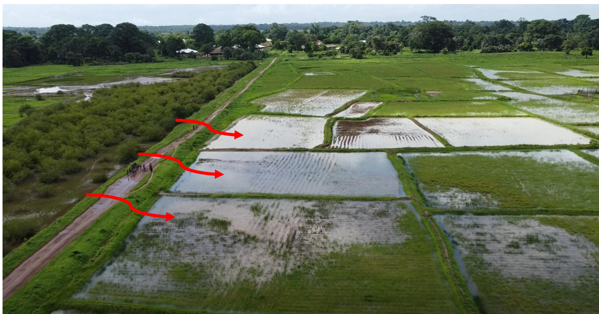
Figure 2: Spatial location of adjacent plots and the potential infiltration of saline water during high tide events.
